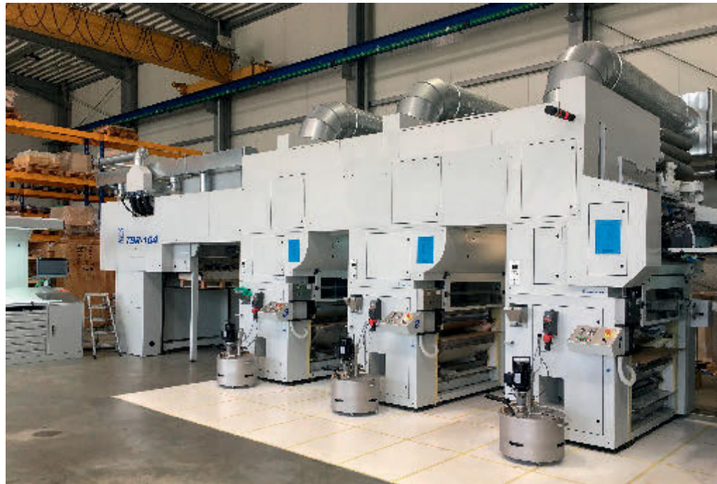
Tatiana Chaykina The new type of sheet-fed press with UV, IR and hot-air drying unit
