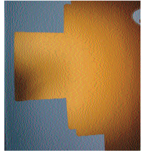
Gravure printed gold for a gloss base, followed by offset printing of images for chocolate packaging, for example.
